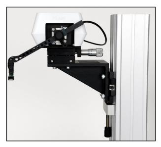
The dimensions of the Piuma Chiaro indentation tips can be varied over several orders of magnitude, covering the whole range of scales that are relevant in tissue engineering and soft (bio)material research. Just plug in the probe, use the microscope to identify the feature or region you want to have information on, and click the start button!
